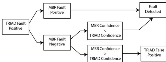
**Figure 5. Diagram of the MAIFLOWER false positive detection system**
