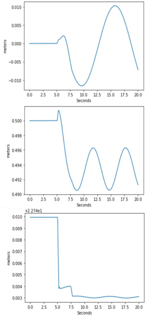
**Figure 7. X (top), Z(middle), Y (bottom) positions of the ROSA tip after the asymmetric soil collapse. The damping coefficient was set to a very low value in the simulation. The initial shorter peak in the first sub-figure represents the initial fall.**
