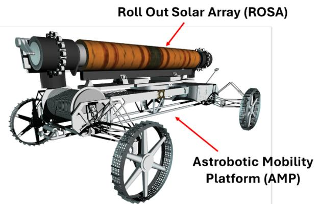
Figure 2. VOLT in stowed configuration<sup>2</sup>
