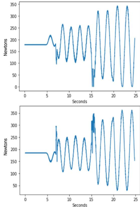
**Figure 10. Normal force exerted on front (top image) and back (bottom image) wheels in the symmetric slipping scenario.**
