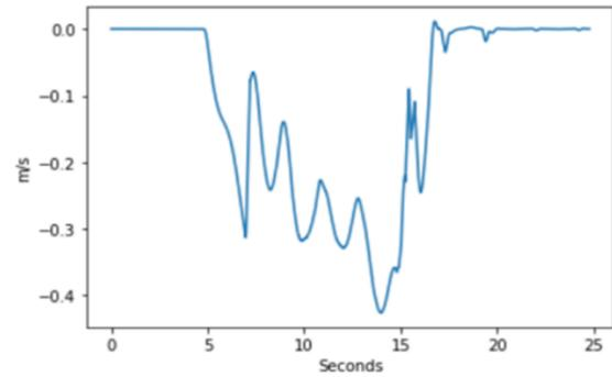
**Figure 9. Y component of velocity in symmetric slipping scenario. The negative velocities occur because the slope goes downward in the -Y direction.**
