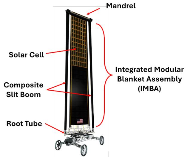
Figure 1. VOLT in deployed configuration<sup>1</sup>
