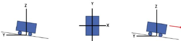
**Figure 8. Sketch of soil slipping scenario, which labels the X, Y, and Z axes and shows the direction of slipping with the red arrow in the right most sketch**
