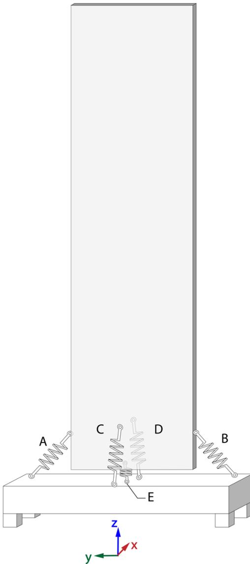
**Figure 6. Spring based model with coordinate reference shown at the bottom**
