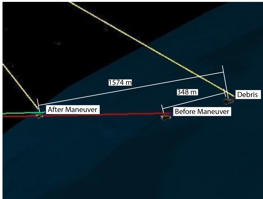
Figure 2. Visualization of the position of the space debris and the satellite after the maneuver and if the maneuver did not happen. Note this image is a screenshot of the 3D GMAT software with some additional overlays to show distances in 3D space. The 2D distances in the image are not to scale with distances in 3D space.
