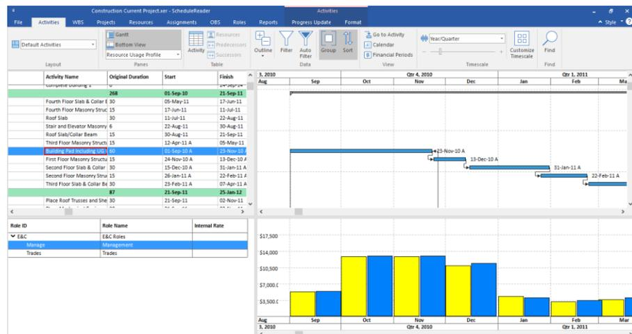
**Trace Logic** and **Resource Usage Profile** view are special views that are always combined with the Activity view. Trace Logic is a very useful view for detail analyzes of a specific portion of the project plan, where users can see the immediate predecessors and successors of a particular task,
