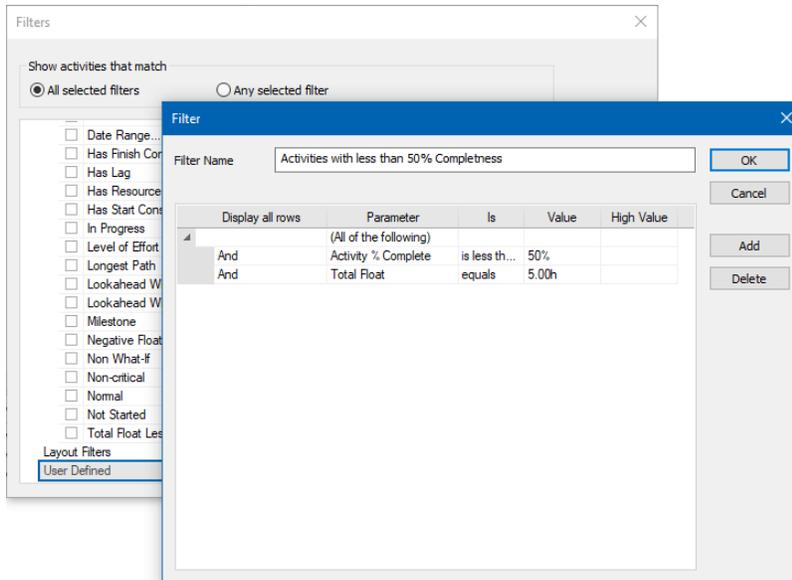
**Filters** are very useful because you can get the required information in a fraction of second. During project execution, you will need filters with complex definitions and filtering criteria. With ScheduleReader™ you can create user-defined filters, that will include or exclude activities in the view, based on the criteria that you specified. **User-defined filters** are saved on the application level, i.e. you can use them in any project plan.
