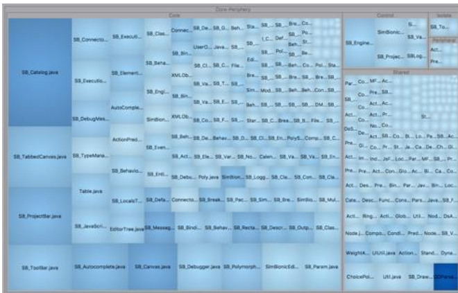
Figure 3. A tree map in Understand where the map is divided by architecture partition, the size of each component is determined by LOC, and color indicates the amount of WMC-McCabe complexity (darker blue is more complex).
