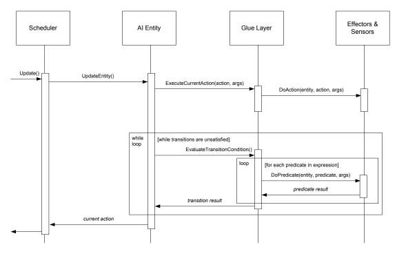
Figure 2- Sequence Diagram of Entity and World Interface
