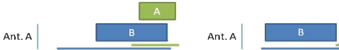
Figure 1: Swapping example (horizontal lines represent view periods) Left: Initially A and B cannot be scheduled because B is using the antenna for too much of A's view period. Right: Schedule A in its view period anyway and B rescheduled.
