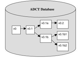
To support concurrent design, ADCT supports a branching model for storing multiple versions of all designs. Any user can split a branch off a previous version. Users can designate any version as their current working version, and so long as that version is unlocked they can perform edits that register in that version. Each version only records its differences from prior versions.
